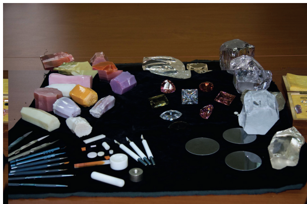
Figure 3 Crystals of phanites, C-OX and PSZ and some articles made thereof.
