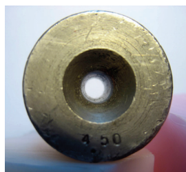
Figure 8 Photograph of a draw plate with profiled PSZ die for producing aluminum and copper wire.
